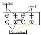
You may not simply remove the thermostat or it will stop running. (Wiring diagram)
