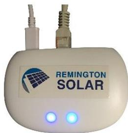
Start with connecting the Hub to your internet router using the provided cable and power. When it is properly connected, power indicator light and internet connection light should stay steady bright blue. If one of them is flashing red, unplug the power of your router and controller, wait for 10 seconds and plug them back in to help bypass the firewall.
